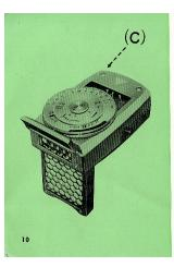
For dim conditions, OPEN the cover, release Booster, by pushing the button, pull up until Booster clicks in place, then use black MARK "\_\_\_\_\_" Center same over the red dot on disk.
