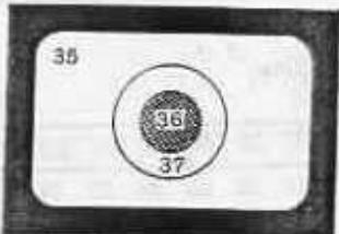
The camera viewfinder is provided with Fresnel lens 35 with two focusing devices in its centre: microraster 36, arranged in the centre of the field, and ground glass collar 37. Watching an object to be photographed, turn the focusing ring to obtain a sharp image on the microraster 36 or the ground glass collar. Focusing is better done at full aperture. The best sharpness is obtained when the image on the microraster is clear, without ripples.
